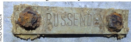
The Russenden cave tag - showing the extensive corrosion of the bolts after a period of submersion. These tags are beautiful and it is very sad to see them falling apart.
