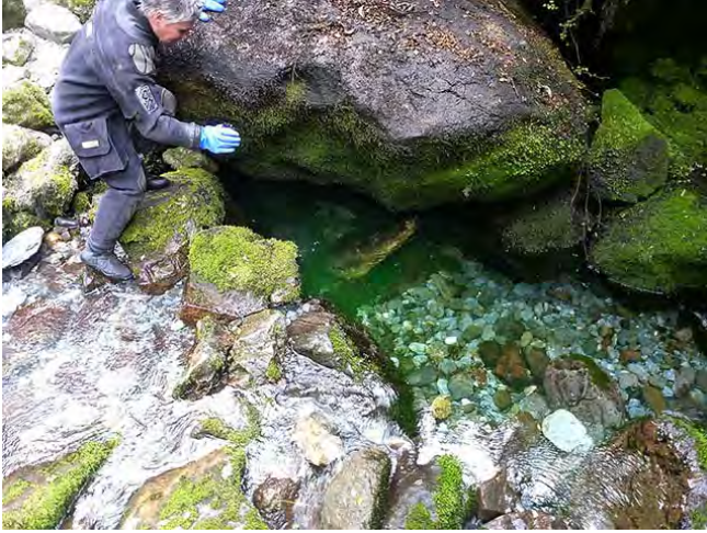
Sandy Varin observes the fluorescein dye emerging from “Mike’s Rear Entrance”. Ken Smith is releasing the dye from about 12m depth.
